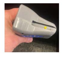
While alcohol-based disinfectants can craze the instruments plastics, we believe that using an alcohol-based disinfectant may be one of the better options for disinfecting your instrument.
