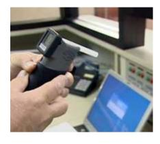
The Alco-Sensor FST and Alco-Sensor  $V_{XL}$  products have two nipples that a mouthpiece attaches to. The mouthpieces are effectively the entire sample path. The mouthpiece for these instruments are designed to direct the breath out the top of the mouthpiece.
